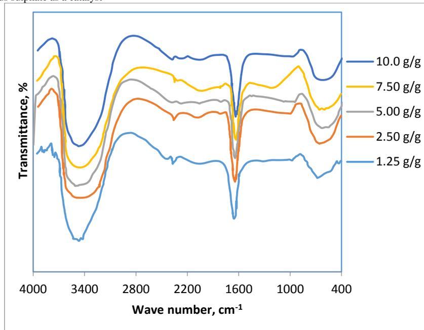
**Fig-8.** IR-absorption spectrum of filtrate resulting from oxidative degradation of protective clothes by H<sub>2</sub>O<sub>2</sub> in presence of different concentrations of copper sulphate as a catalyst
