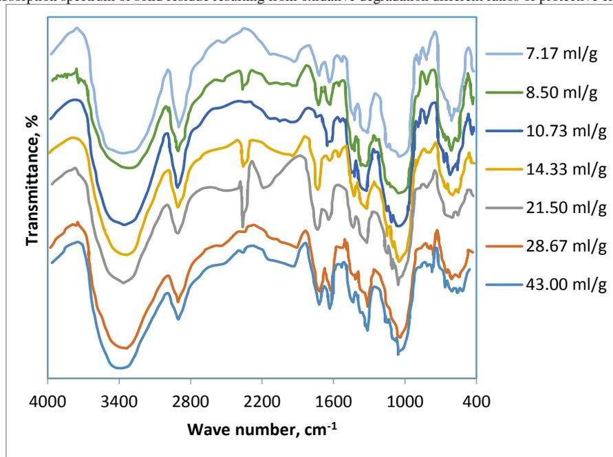
**Fig-4.** IR-absorption spectrum of solid residue resulting from oxidative degradation of protective clothes by  $H_2O_2$  in presence of different concentrations of ferrous sulphate as a catalyst
