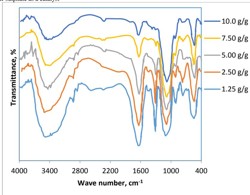
**Fig-6.** IR-absorption spectrum of filtrate resulting from oxidative degradation different ratios of protective clothes by H<sub>2</sub>O<sub>2</sub>
