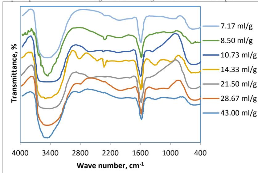
**Fig-7.** IR-absorption spectrum of filtrate resulting from oxidative degradation of protective clothes by H<sub>2</sub>O<sub>2</sub> in presence of different concentrations of ferrous sulphate as a catalyst
