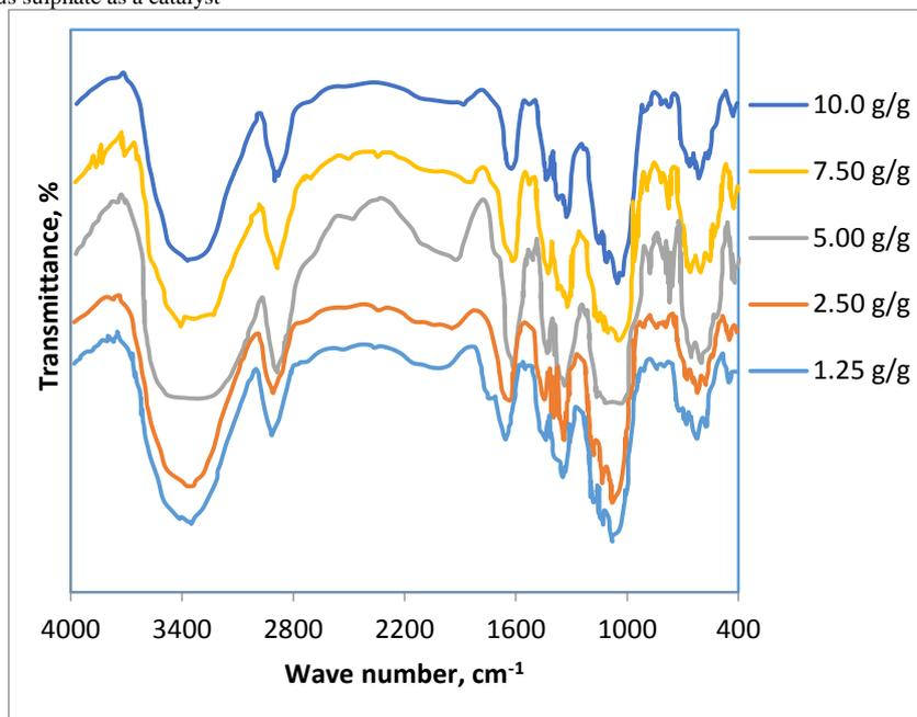
**Fig-5.** IR-absorption spectrum of solid residue resulting from oxidative degradation of protective clothes by  $H_2O_2$  in presence of different concentrations of copper sulphate as a catalyst
