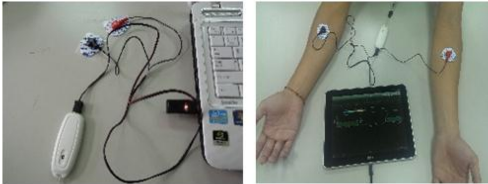
Fig-2. Self-developed two pole ECG acquisition device.
