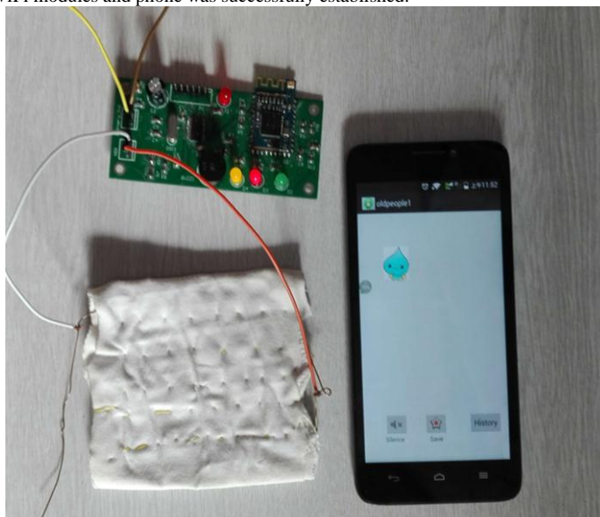
Figure-6. Illustration of simulation. device is shown in the picture. The yellow light shined when WiFi modules work well. The red light shined when TCP connection between WiFi modules and phone was successfully established.
