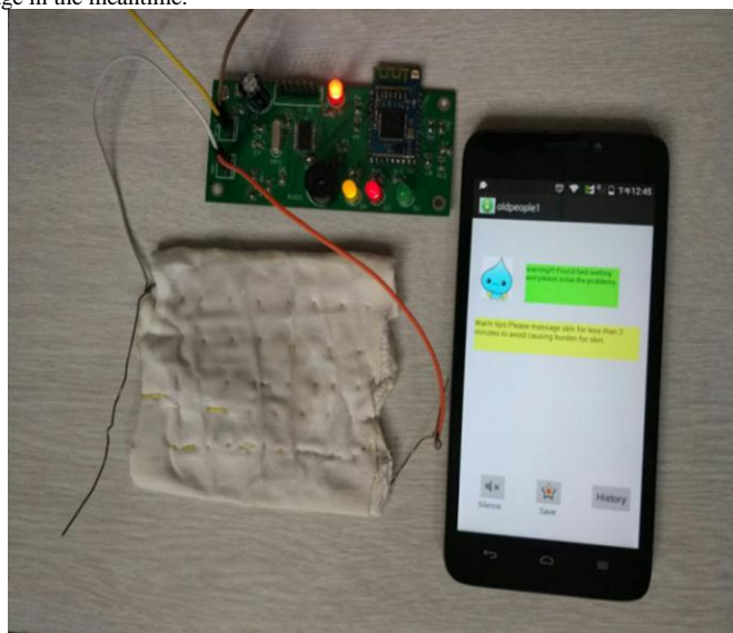
Figure-7. Illustration of alarm. How the alarm signal present is shown in the picture. The alarm light shined and alarm buzzer pealed. The long-range phone showed alarm message in the meantime.
