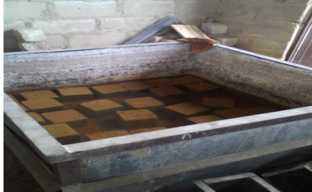
Plate-3. Curing of concrete cubes in water
