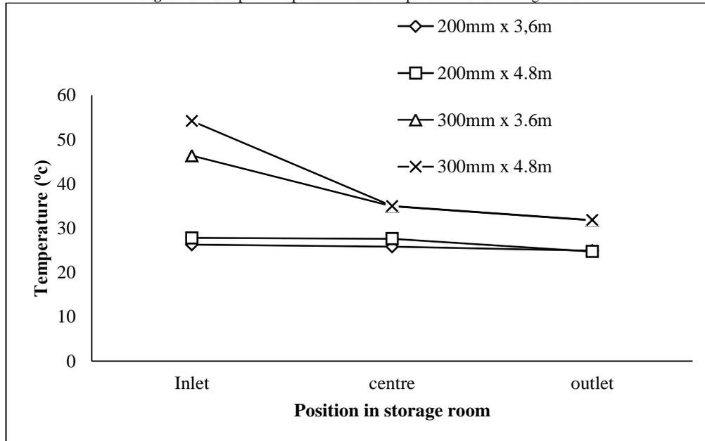
However, for a 200 mm diameter chimney, the temperature does not change, irrespective of the position in the storage room. In principle, the air cools as it sinks in space [31, 41], which implies that a chimney size with a diameter of 300 mm has an ability to circulate the air in the storage room and a chimney with a diameter of 200 mm does not induce air movement in a storage room.
