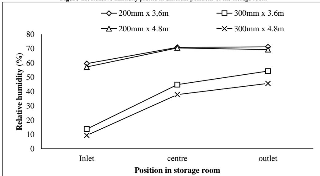
When the temperature decreases, the relative humidity tends to increase, since air with a low temperature has little capacity to hold moisture, resulting in high relative humidity [49-51]. On the other hand, the chimney diameter of 200 mm had a high relative humidity in all the positions in the storage room. This is an indication that the air is still in the storage space, when a chimney diameter of 200 mm is used.
