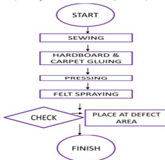
Fig-1. Process Flow Chart of the Car Carpet Assembly line.
