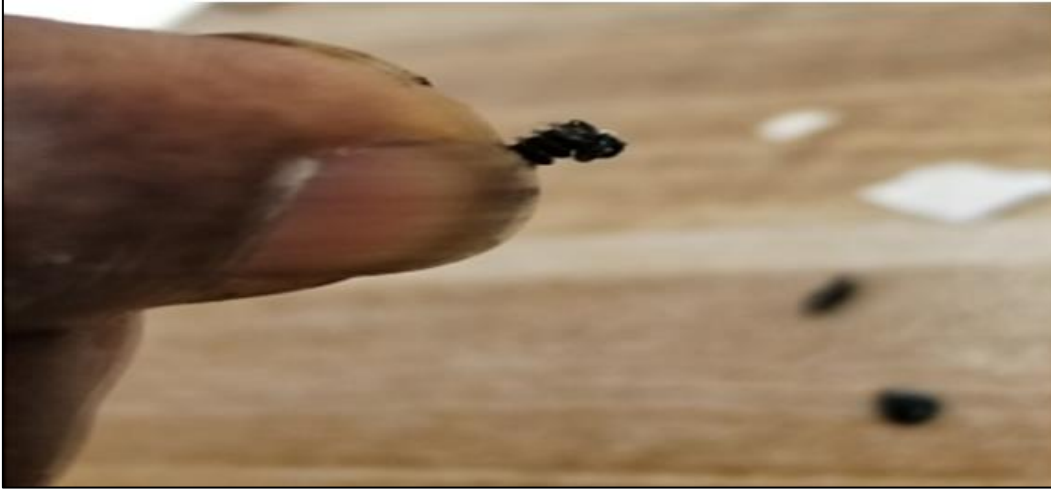
Figure-4. Attraction of a sample of ammonium sulphate by a screw
