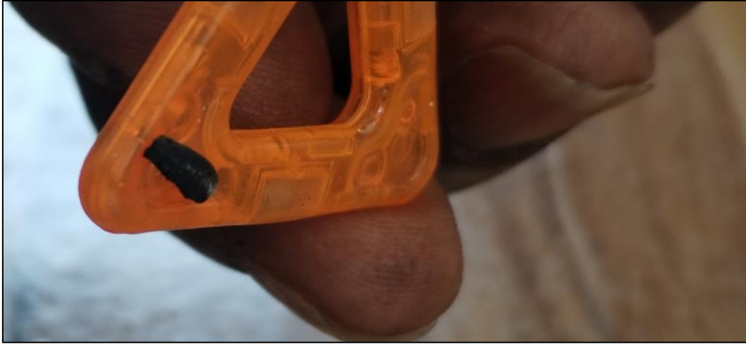
Figure-5. Attraction of a sample of ammonium sulphate by a magnet
