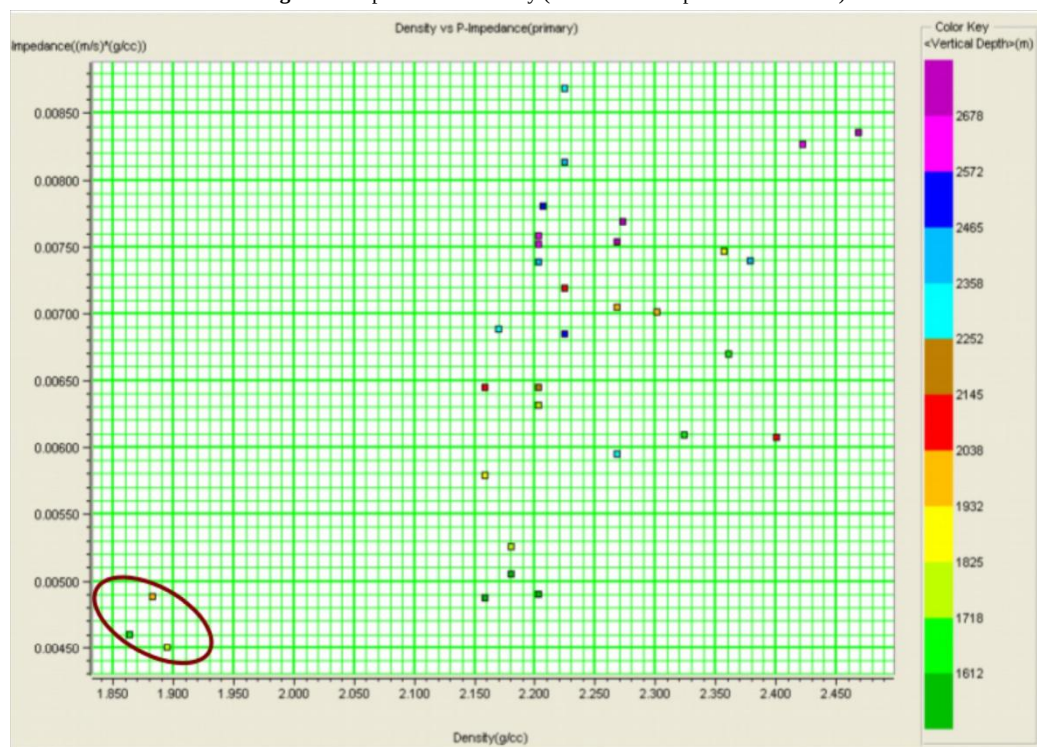
Fig-4b. P-impedance vs Density (with vertical depth as colour code).
